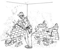
It may also be useful to remove the plaster at least at one side of the walls from the floor up to some centimeters above the highest level of the water. Especially consider removing the plaster if the wall contains wooden elements, which may rot if not dried properly.
